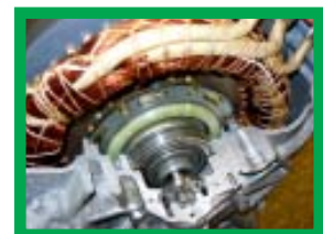
MGU- Motor/Generator Unit
