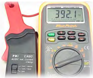
Non-intrusive Amperage Testing
